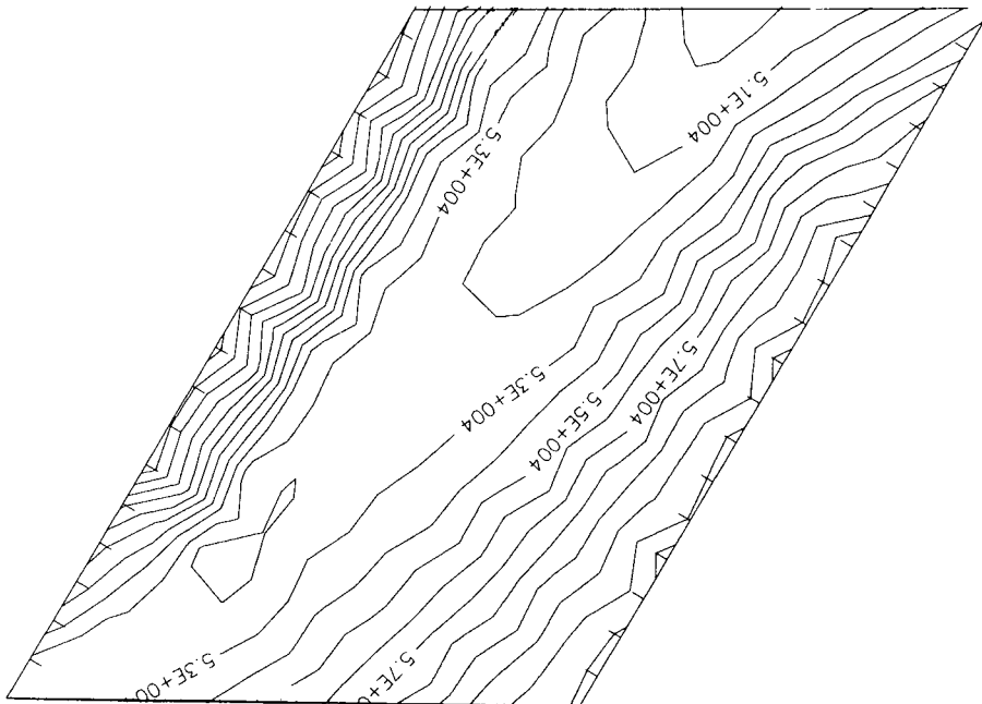
Figure 27. Current-method-predicted isobars on the blade surface of the 30° swept aerofoil at p_2/p_{01} = 0.623
